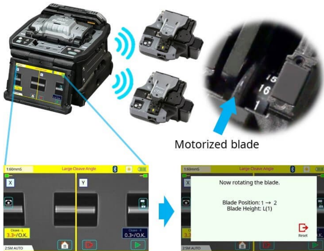
Figure 1- Automated fiber alignment, Bluetooth communications and real-time arc control reduce the skill and time required to produce high quality splices.
