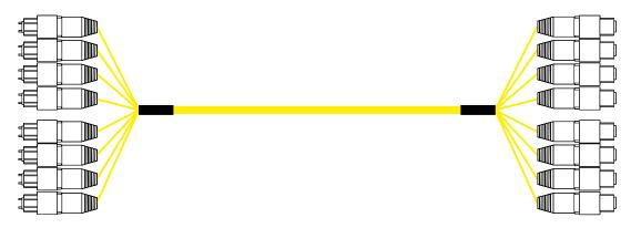
A cross between a shuffle patchcord and a shuffle trunk, a high-count patchcord combines two or more 32f mesh units into a single patchcord type assembly. A trunk patchcord could be deployed in the same rack or in the same row of a data center but should not be used as main infrastructure running down the length of the data center.
